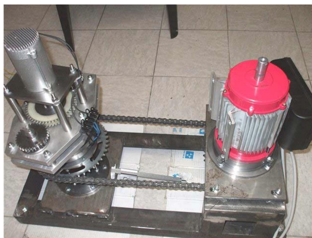
Fig. 4. Model of a drive of a rotor of the electrogenerator (on the right) power of 6 kWatt the electric motor (at the left) power of 500 Watt (Austria, January 2009.)
